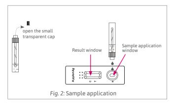
5. Read results at **10 minutes** after dispensing the specimen. Do not read results after 20 minutes.
